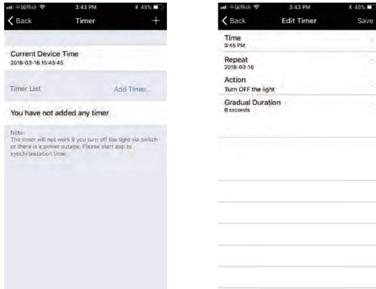
The controller has a build in timer function. To do so, press on the top right, next to ON/OFF, switch the clock icon. Then the selection menu will be shown with time, Repeat (Mon-Sun), ON/OFF switch and the optional Model (color setting, Brightness and gradient program.) The timer will not operate when the power supply is interrupted. In this case, start the APP to resynchronize.
