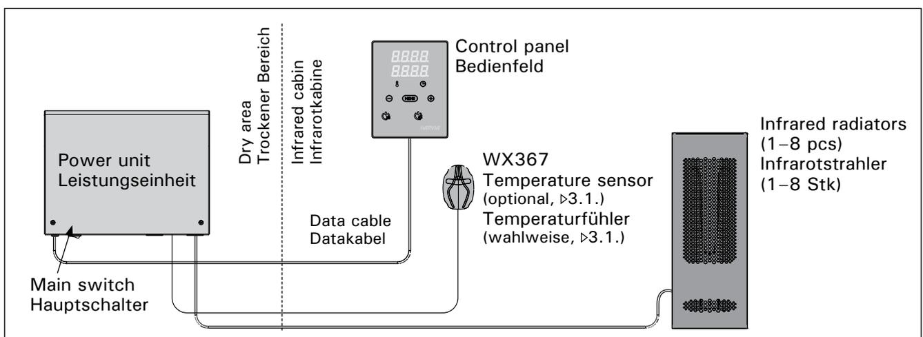
Figure 1. System components
