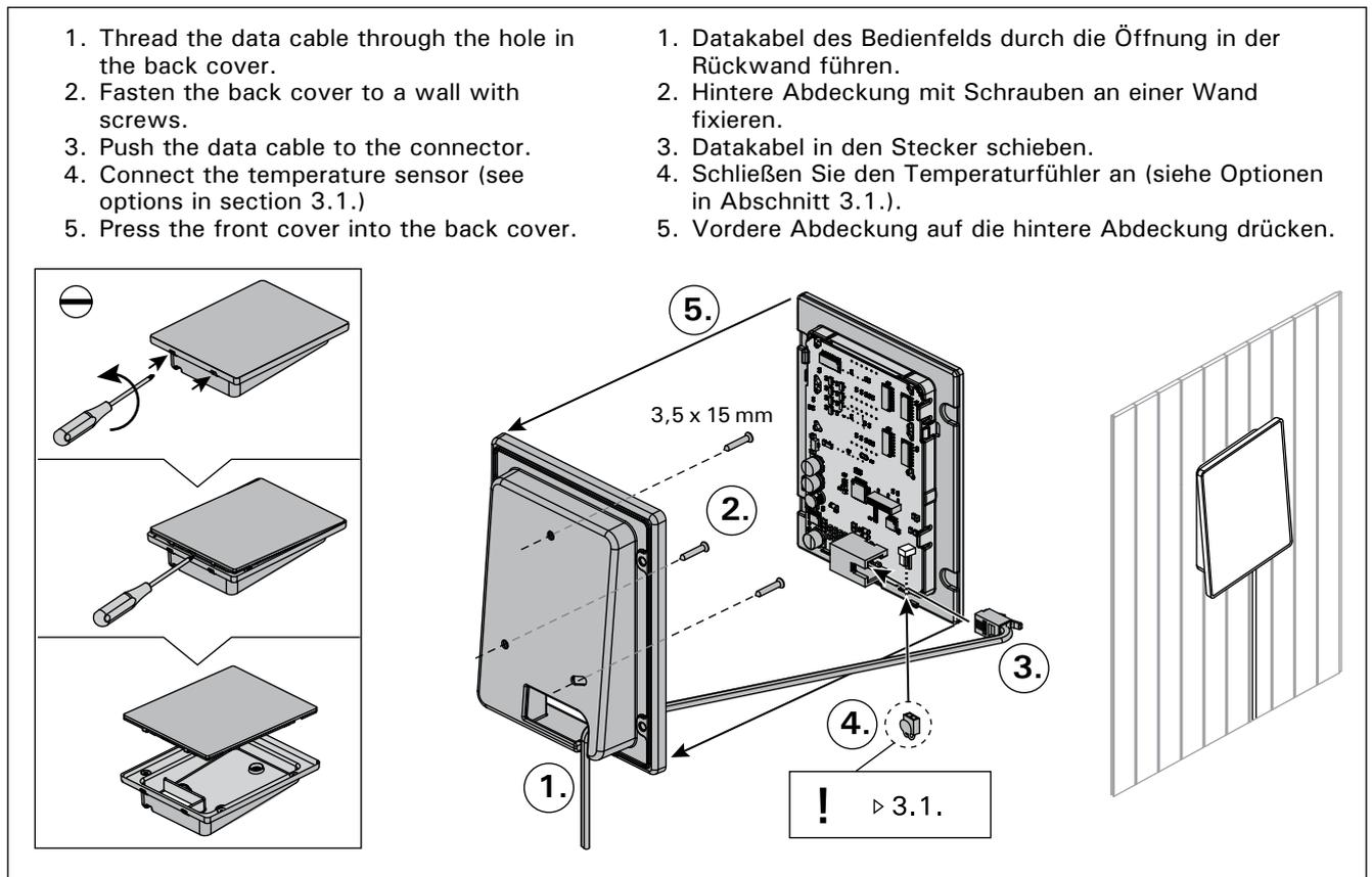
Figure 9. Fastening the control panel
